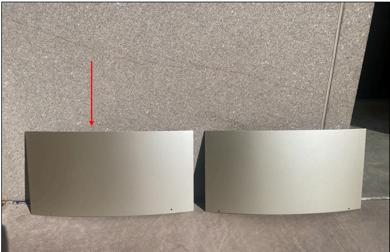
5 6 BLC Addition metal cladding finish samples, placed against Colonial Rose granite on the NASM building, 7 February 2025. Selected finish (Titanium) at left, noted with a red arrow. 8
