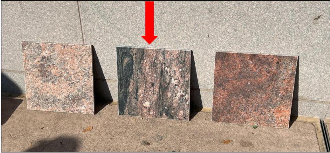
Left: Coldspring Agate Granite with diamond 10 finish; Center: Coldspring Rainbow granite with diamond 8 finish; Right: Coldspring Agate Granite with diamond 8 finish. Samples are laid against the Colonial Rose that will be used in the site walls to match the larger NASM site. (EHT Tracerics, 2024)
