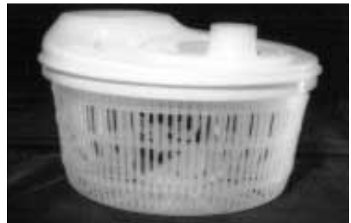
Apparatus assembled. Turning knob on top will make cage spin.
